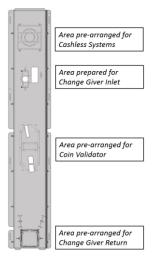
The machine is prepared for payment. The payment kit is applicable for both the Coin Changer and Coin Validator system and has an area pre-arranged for Cashless Systems. Please order additionally the black poster which is available when using the Coin Changer, to avoid using the standardized poster of the supplier. A black poster for the Coin Validator has been requested as well.
