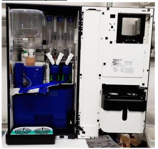
Due to the brewing type, the FresBrew OMNI has the availability of standard 3 canisters. This can be extended via a 4<sup>th</sup> canister, similar to the B2C variants of the OMNI, but due to expected low numbers, these recipe files will only be created for a large request.
