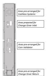
The machine is prepared for payment. The payment kit is applicable for both the Coin Changer and Coin Validator system and has an area pre-arranged for Cashless Systems. Please order additionally the black poster which is available when using the Coin Changer, to avoid using the standardized poster of the supplier. A black poster for the Coin Validator has been requested as well.
